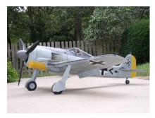
long as the epoxy paint is not flooded on. You can't get the latex too wet with anything that has acetone or toluene in it. These chemicals turn the latex to a rubber cement kind of goo. On the second FW-190 I used latex for all the colors including all the camouflage and markings. The first FW-190 had a coat of satin clear epoxy over the latex, the second FW-190 had no clear coat on it. In my opinion the second one came out better.
