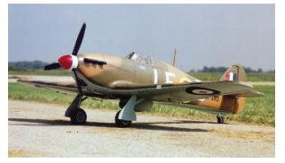
latex applied directly to the "raw" Coverite. The latex took to the Coverite like it was made especially for it. Great.... Nice thing here was that even when the fabric sags or takes a dent you can apply heat and re-shrink the fabric and the paint just goes along for the trip. Another thing I discovered is that latex paints don't crack due to vibration or expansion / shrinkage of parts. It's rubber, right....
