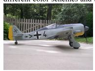
great results. On the first Focke Wulf I used latex for the base color and all the camouflage but used epoxy paint over the latex for the markings. (The Thunderbolt and the Hurricane also used this treatment). This works ok as
